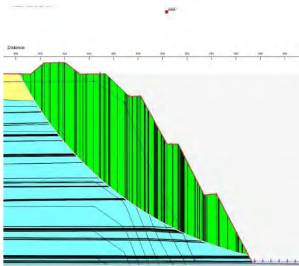
Figure 5-9 Low Strength Model Full Depth \ Pit RHS
